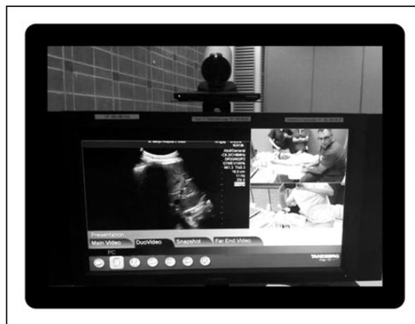
**Figure 1.** Telemedicine equipment at St. Mary's Hospital Center. Two Cisco Edge 95 MXP videoconferencing devices were connected point to point at a data transfer rate of 768 kbps over IP network using H.323 protocol. The ultrasound systems video outputs were transmitted using the presentation channel (duo video).
